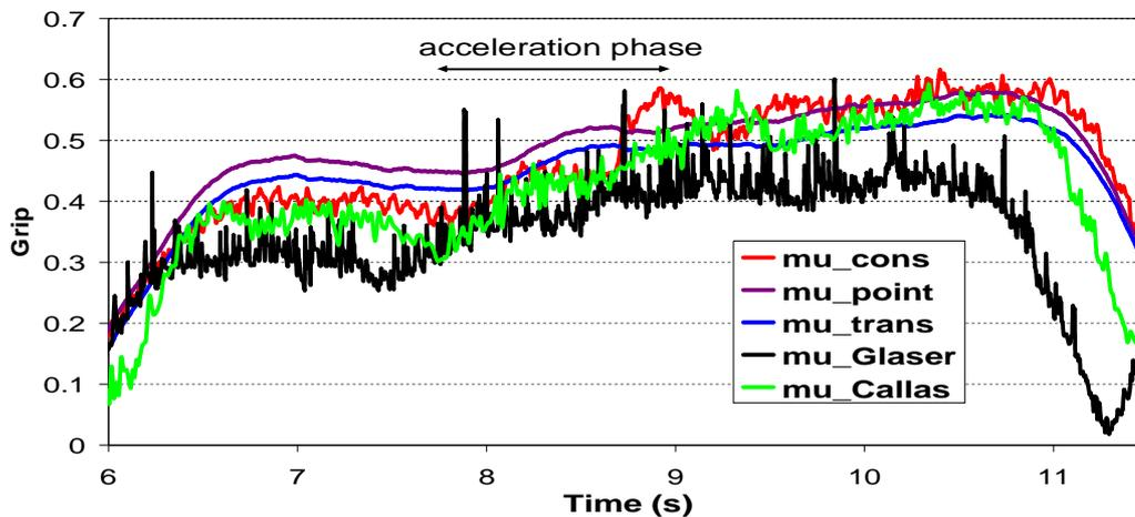
Figure 7. Consumed grip,  $v=80\text{km/h}$ ,  $r=110\text{m}$ , dry surface, acceleration
