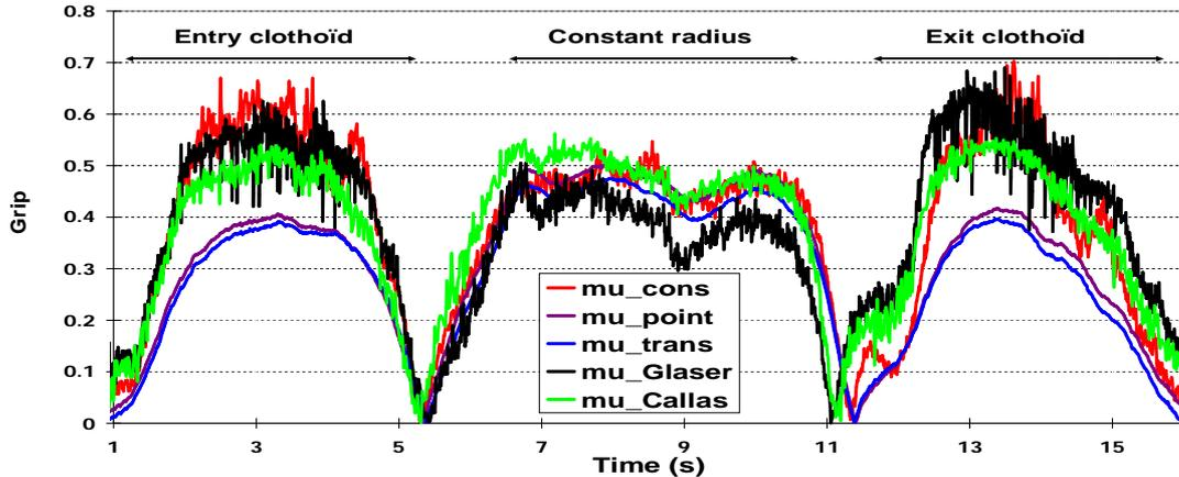
Figure 6. Consumed grip,  $v=82\text{km/h}$ ,  $r=110\text{m}$ , wet surface
