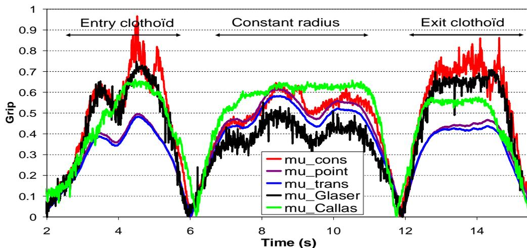
Figure 5. Consumed grip,  $v=88\text{km/h}$ ,  $r=110\text{m}$ , dry surface
