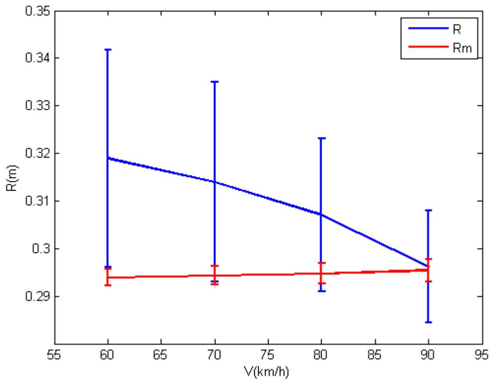
Figure 5. Radius evolution with vehicle speed in the 110 m curvature corner
