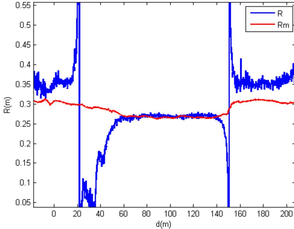
Figure 3. Measured ( $R_m$ ) and deduced ( $R$ ) radii for a road radius of 90 m at 90 km/h.
