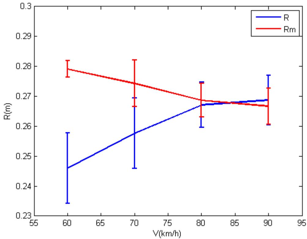
Figure 4. Radius evolution with vehicle speed in the 90 m curvature corner
