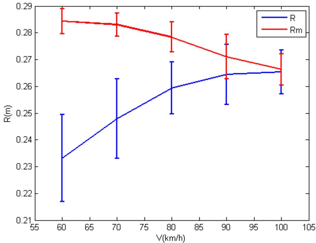
Figure 6. Radius evolution with vehicle speed in the 130 m curvature corner
