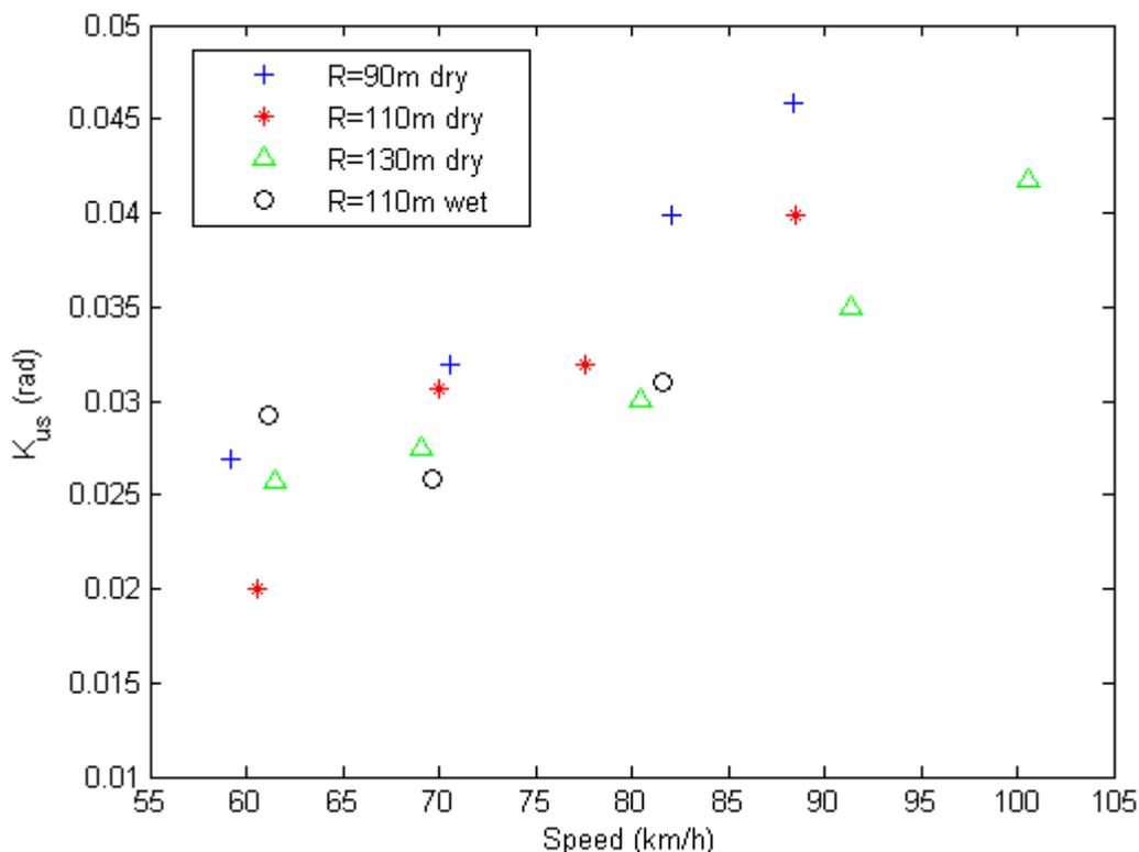
Figure 2-Understeer gradient versus speed
