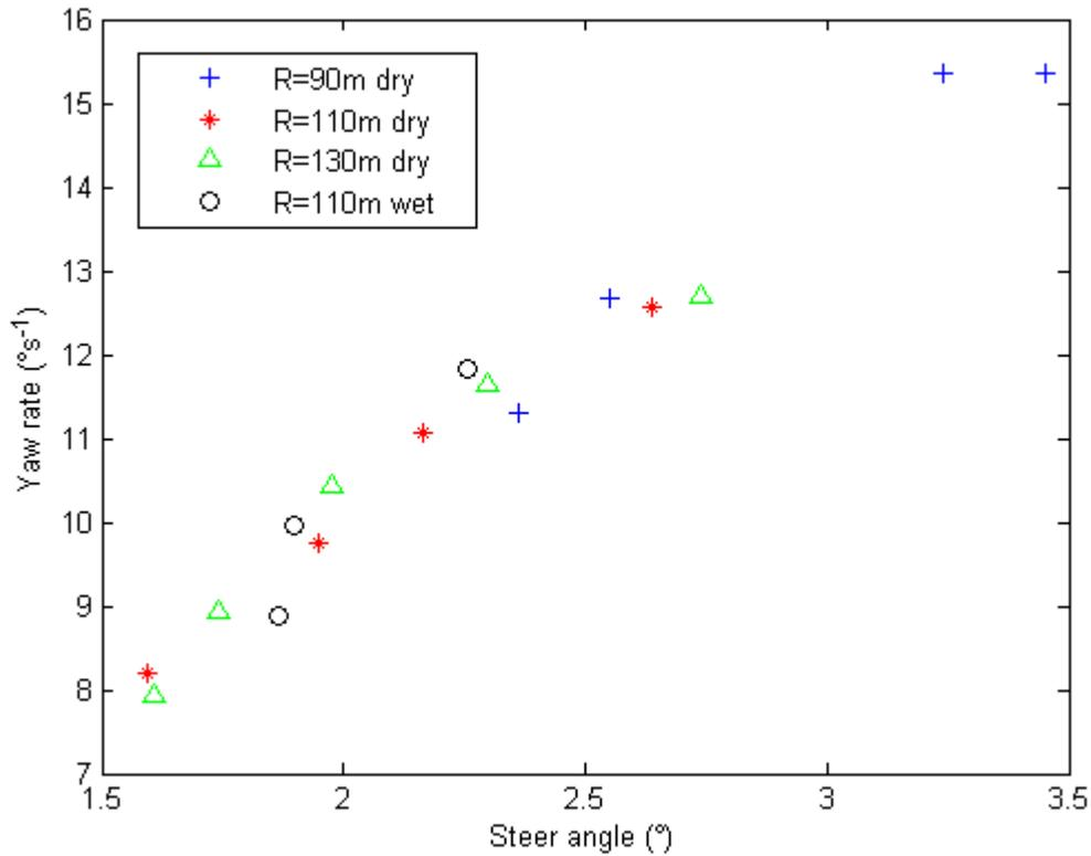
**Figure 3- Yaw rate versus steer angle**
