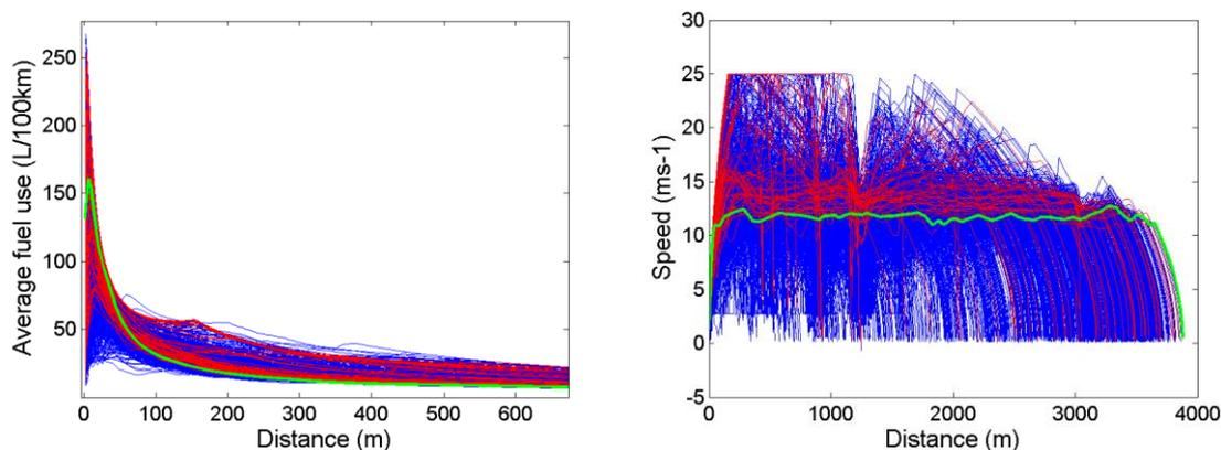
**Figure 5 – Left: Cumulated fuel consumption; Right: Speed profiles for all drivers during the Paris Motor Show Paris. Blue: All profiles; Red: Optimal profiles (Pareto definition); Green: Best profile**
