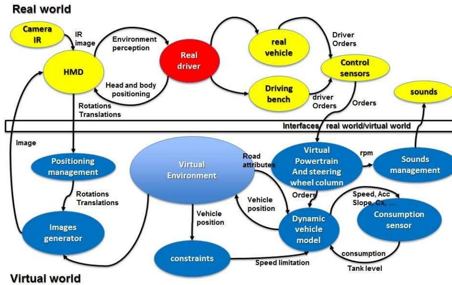
**Figure 3 - Functional diagram of the eco-SiVIC platform**
