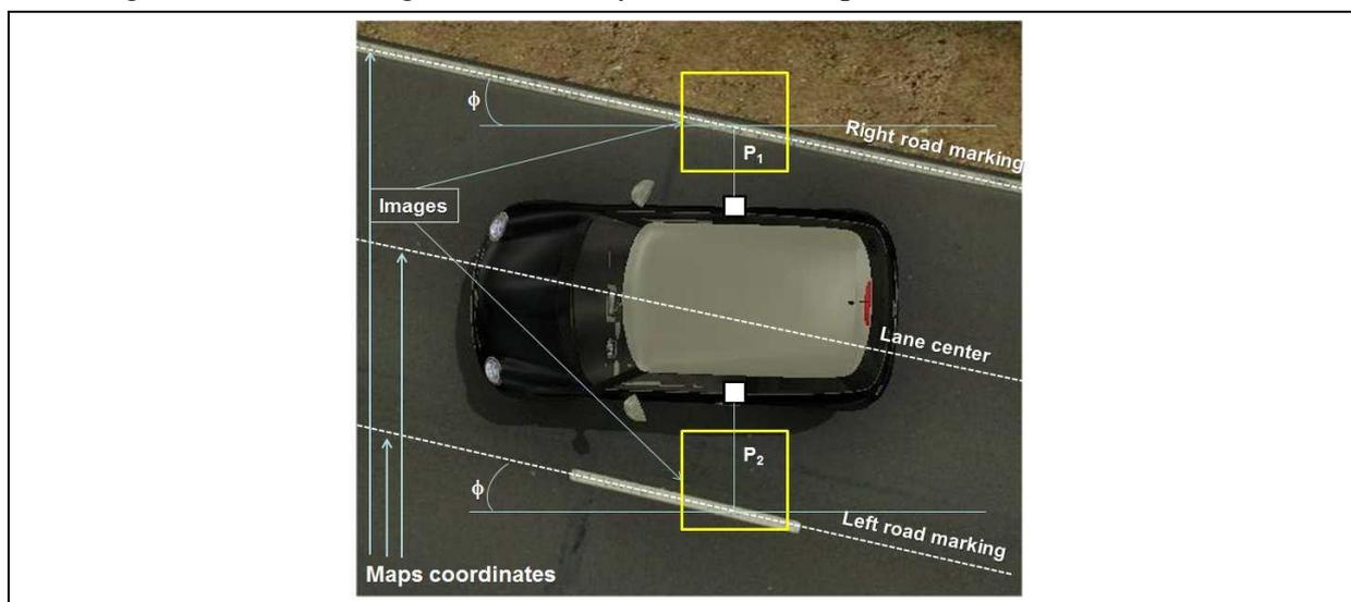
Figure xx: Ego-positioning enhanced with road marking detection and accurate MapMatching processes.
