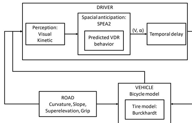
**Figure 1: Synthesis of Evolutionary Multiobjective Optimization Trajectory Planning Algorithm**
