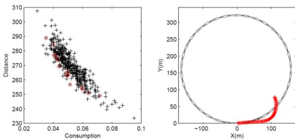
**Figure 2: Construction of Pareto frontier: Left, Pareto frontier in red, all solutions in black; Right, an unsafe trajectory.**
